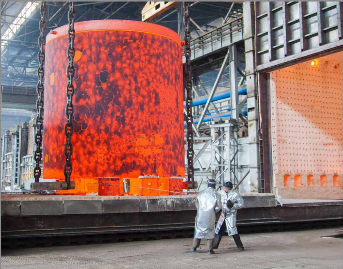
Hardening of VVER-TOI shell - Energomashstal JSC
